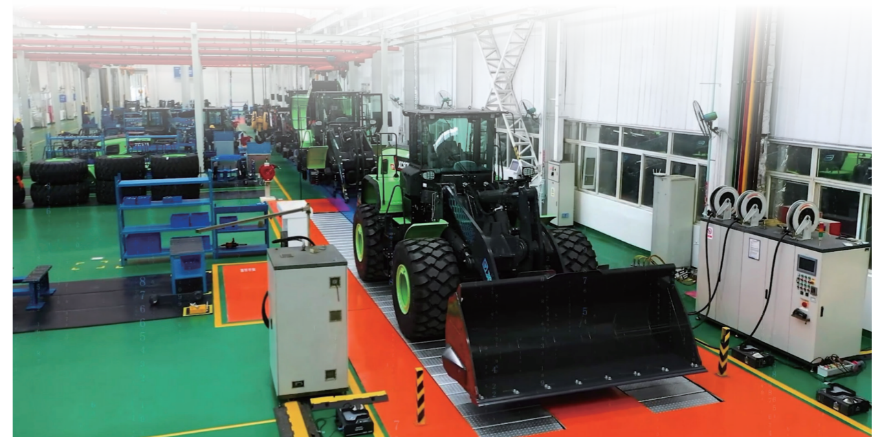
▲ In November 2023, the world's first electric loader production line, which produced the XC988-EV, the largest-tonnage electric loader across the world, was put into operation at XCMG. Every 25 minutes, an electric loader is off from this production line.
