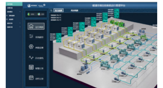
Air conditioning smart control management system
